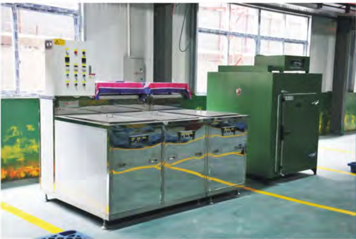
脱脂装置 Degreasing Plant
